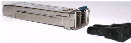
Figure 6: SFP module and optical port plug
